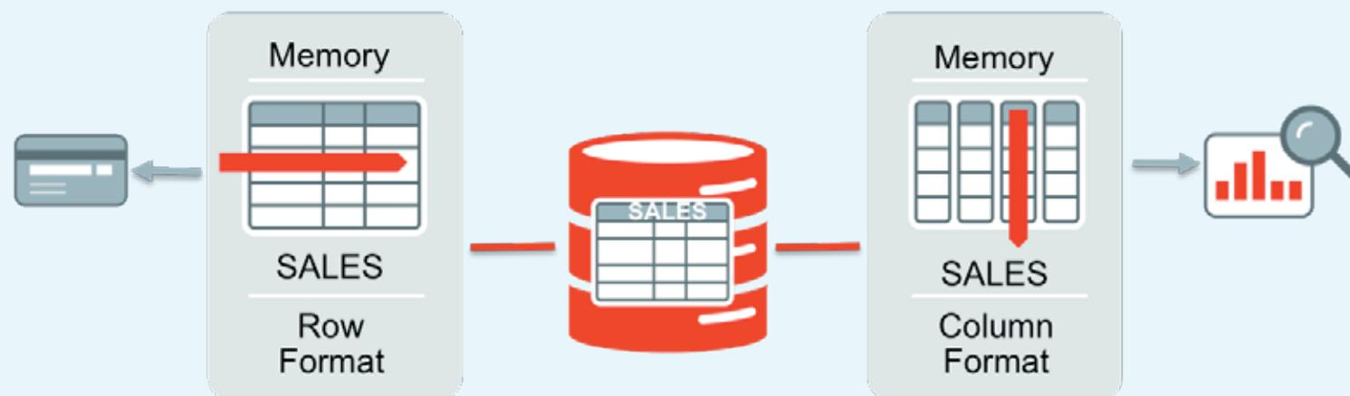
Figure 2 Oracle's unique dual-format in-memory architecture
