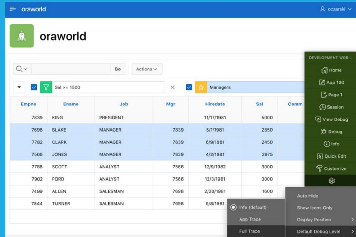
Fig. 1: Use the Developer Toolbar to toggle the debug level.
